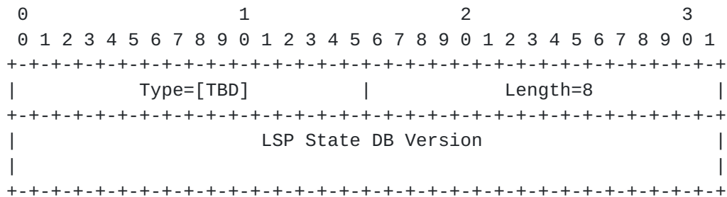
Figure 15: LSP-DB-VERSION TLV format
