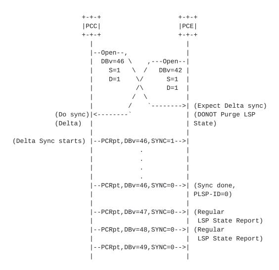
Figure 7: Incremental Synchronization Procedure
