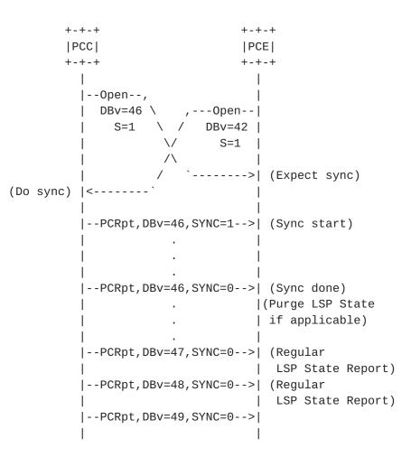
Figure 2: State Synchronization Performed
