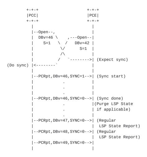
Figure 2: State Synchronization Performed
