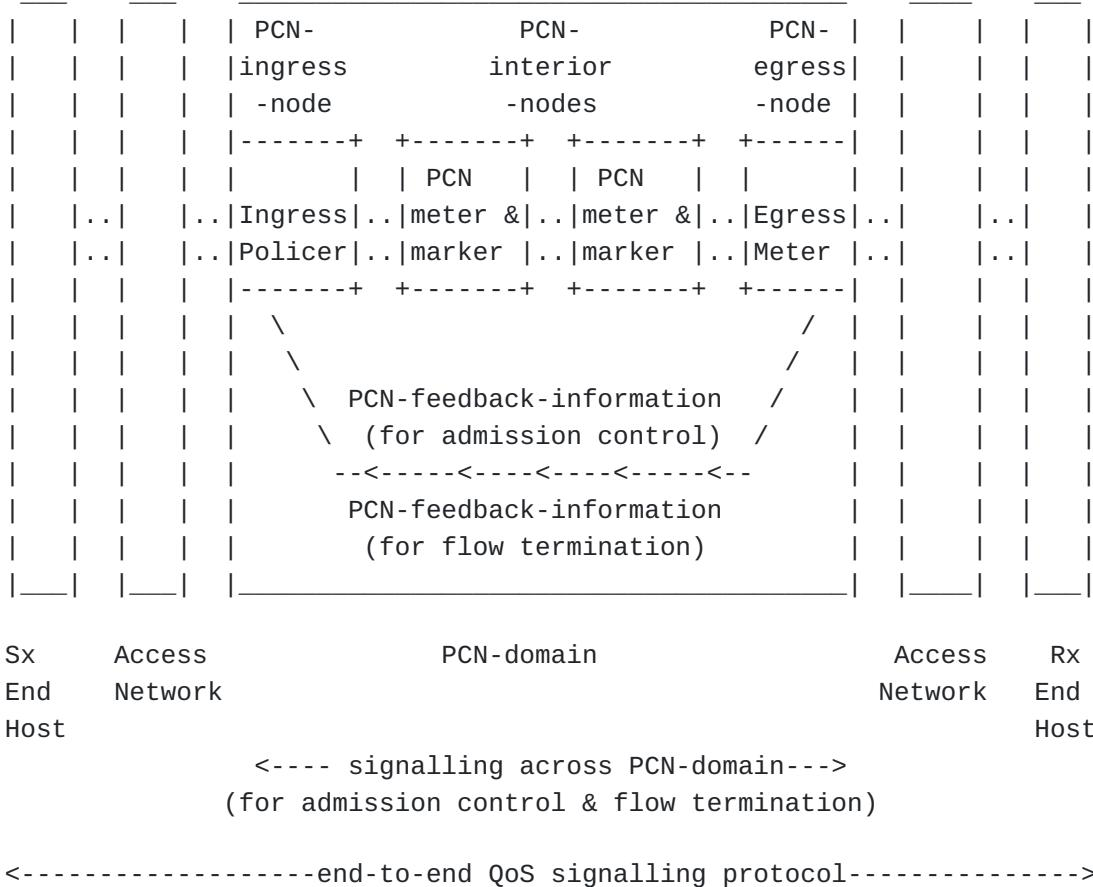
Figure 2: Example of possible overall QoS architecture
