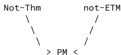
Figure 3: PCN Codepoint Re-Marking Diagram for Packet Specific Dual Marking (PSDM)
