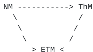
Figure 1: PCN Codepoint Re-Marking Diagram for Dual Marking (DM)
