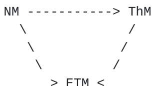
Figure 1: PCN Codepoint Re-Marking Diagram for Dual Marking (DM)
