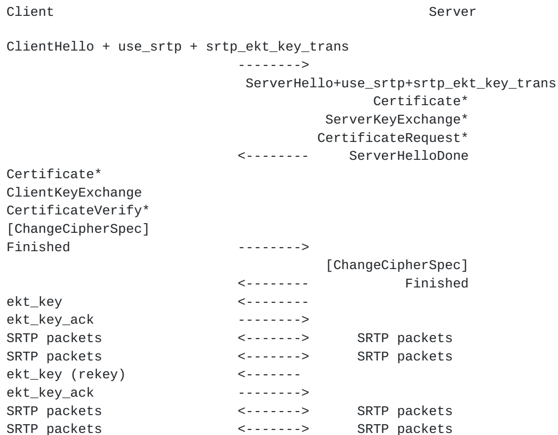
Figure 5: DTLS/SRTP Message Flow
