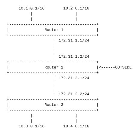
Router 1 can reach its two locally connected subnets, 10.1.0.0/16 and 10.2.0.0/16. It will aggregate them into a single announcement of 10.0.0.0/8 when it advertises out the 172.31.1.1 interface.
