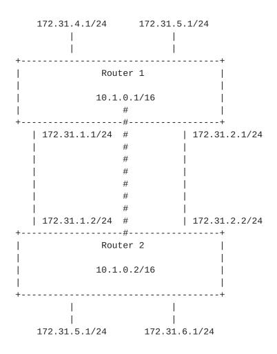
A common practice to provide router identifiers is using the "highest IP address" on the router as an identifier for the "box." Many implementations have a default mechanism to establish the router ID, which may be the highest configured address, or the highest active address.
