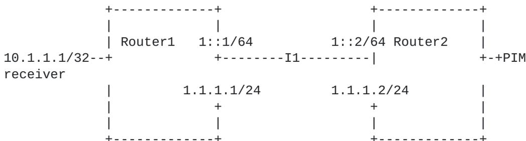
In example topology, Router1 and Router2 are PIMv4 and PIMv6 neighbors on Interface I1. Router2 learns prefix 10.1.1.1/32's
