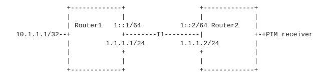
In example topology, Router1 and Router2 are PIMv4 and PIMv6 neighbors on Interface I1. Router2 learns prefix 10.1.1.1/32's nexthop as 1::1/64 on Interface I1 as advertised by Router1 using BGP IPV6 NLRI.But in order to send (10.1.1.1/32, multicast-group) PIMv4 join on Interface I1, Router2 needs to find corresponding PIMv4 neighbor. In case there are multiple PIMv4 neighbors on same Interface I1, problem is aggravated.
