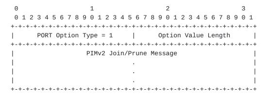
The IPv4 Join/Prune Option is used to carry a PIMv2 Join/Prune message that has all IPv4 encoded addresses in the PIM payload.
