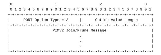
The IPv6 Join/Prune Option is used to carry a PIMv2 Join/Prune message that has all IPv6 encoded addresses in the PIM payload.
