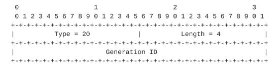
Generation ID is a random 32-bit value for the interface on which the Hello message is sent. The Generation ID is regenerated whenever PIM forwarding is started or restarted on the interface.
