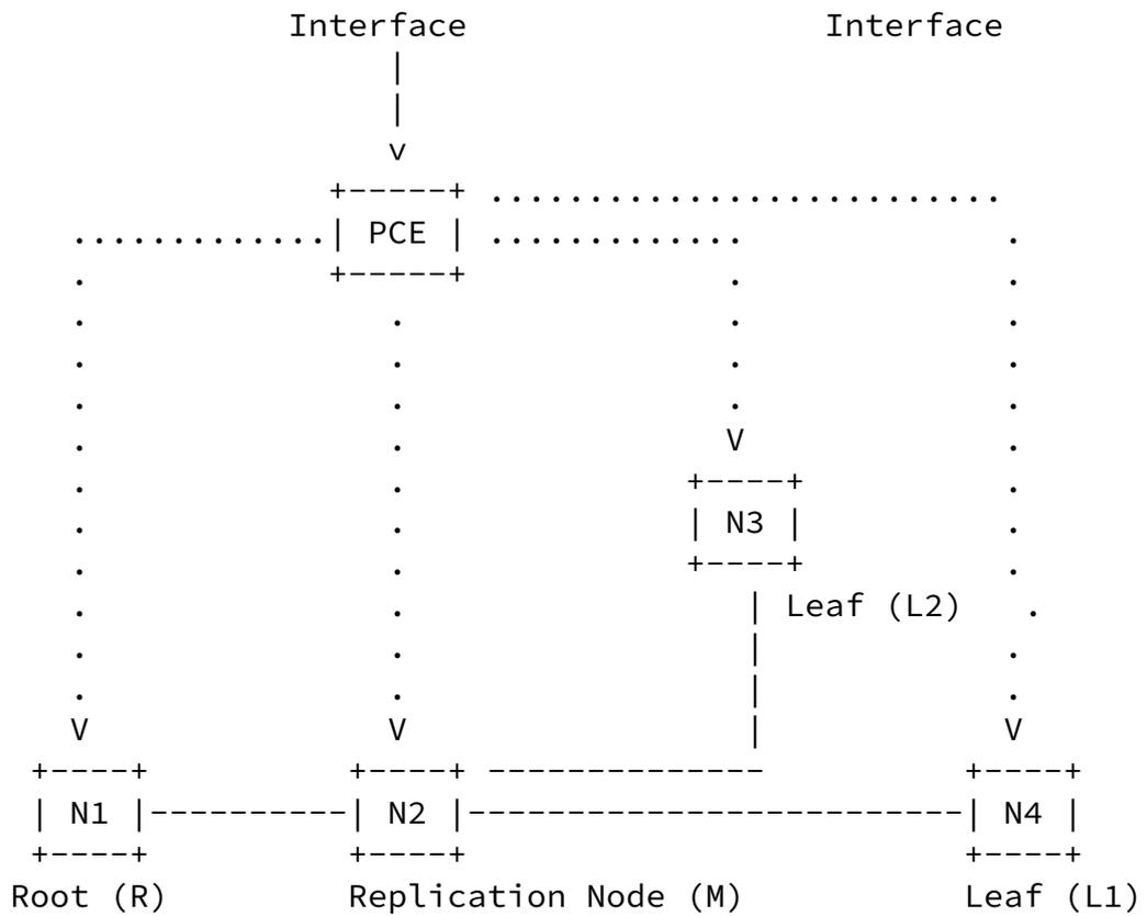
Figure 1: Centralized Control Plane Model
