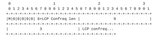
This AVP contains a list of options that the LAC would like to see negotiated by the LNS. In some cases this maps to a desired value (e.g., MRU) and in some cases it maps to a specific option that is desired to be enabled (e.g., ACFC). The LNS should use these suggestions when building its initial Configure- Request. Presence of this AVP is optional.
