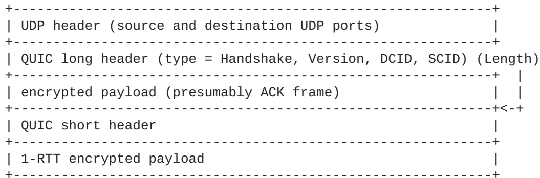
Figure 5: Typical QUIC Handshake Completion datagram pattern
