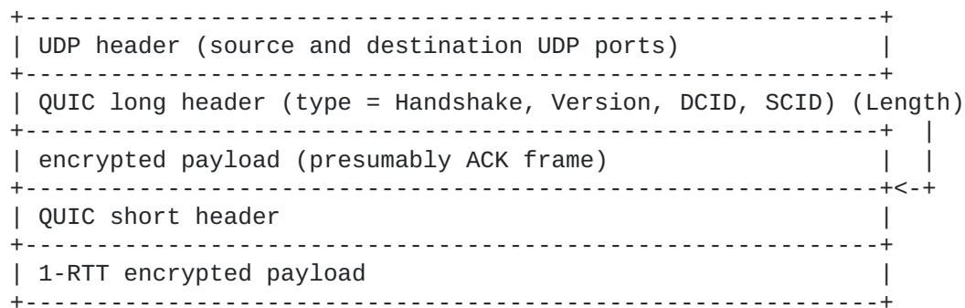
Figure 5: Typical QUIC Handshake Completion datagram pattern
