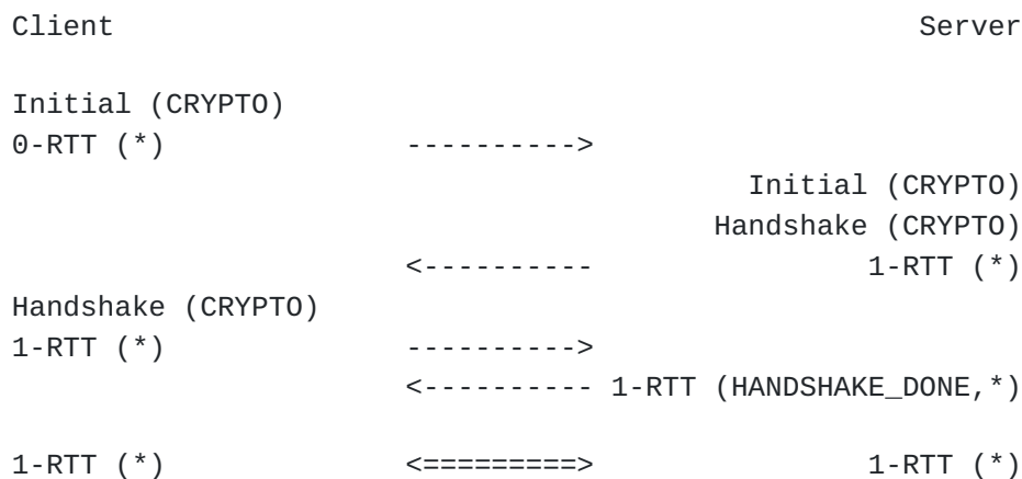
Figure 4: Simplified QUIC Handshake
