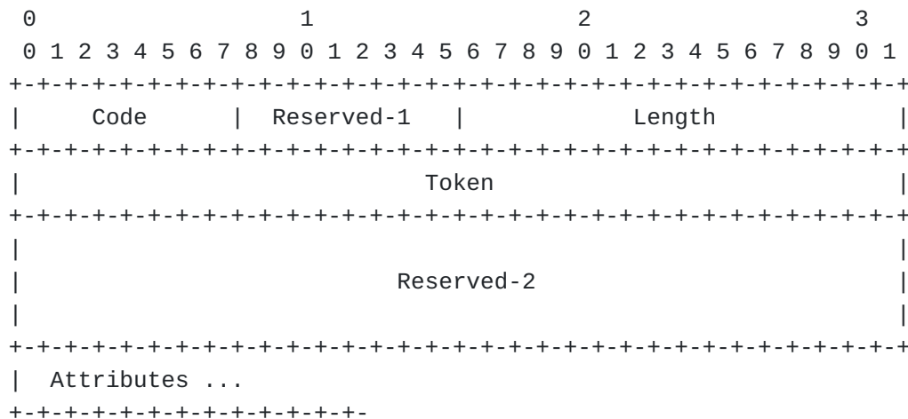
Figure 2: The RADIUS/1.1 Packet Format
