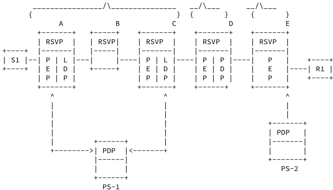
Figure 4: Placement of Policy Elements in an internet
