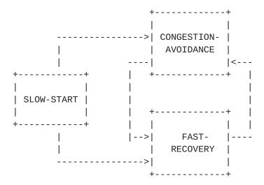
This algorithm (Algorithm ACK) maintains 3 states: SLOW-START, CONGESTION-AVOIDANCE and FAST-RECOVERY, which are equivalent to the states in TCP congestion control algorithms. It also maintains 2 variables: cwnd and ssthresh.
