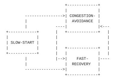
Initially, this algorithm starts in state SLOW-START with ssthresh set to ISSTHRESH and cwnd set to IW.
