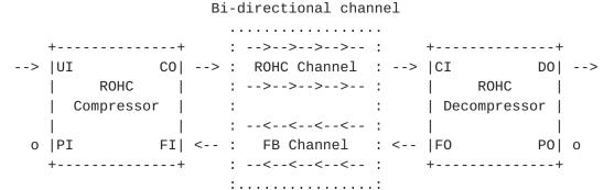
In this example, feedback is sent on its own dedicated channel, as discussed in e.g. feedback realization example 1-3 of ROHC [RFC-3095, page 44]. This means that the piggybacking/interspersing mechanism of ROHC is not used, and the PI/PO connections are thus left open (marked with a "o"). To facilitate communication with ROHC
