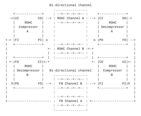
In this example, feedback is in both directions sent on its own dedicated channel, as discussed in e.g. feedback realization example 1-3 of ROHC [RFC-3095, page 44]. With this configuration, the piggybacking/interspersing mechanism of ROHC is not used, and the PI/PO connections are thus left open (marked with a "o"). It should be noted that also in this picture, PO and FO at the decompressors have been swapped to simplify drawing, as well as the B-instances have been vertically mirrored.
