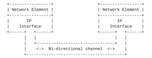
A typical example of a point-to-point link with such a bi-directional channel is a PPP modem connection over a regular telephone line. Header compression can easily be applied here as well, as usually done over e.g. PPP, and the compression scheme can make use of the return path to improve compression performance.
