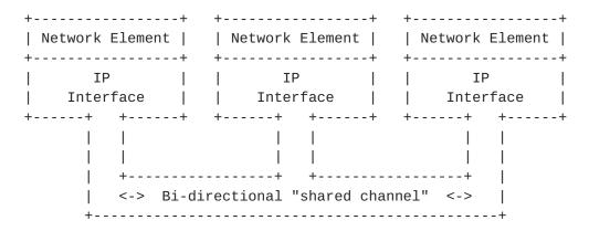
A typical example of a multipoint link with a bi-directional "shared channel" like this is an Ethernet. Since the channel is shared, applying header compression would require a lower layer addressing scheme, to provide logical point-to-point channels, according to the definition of "channels".
