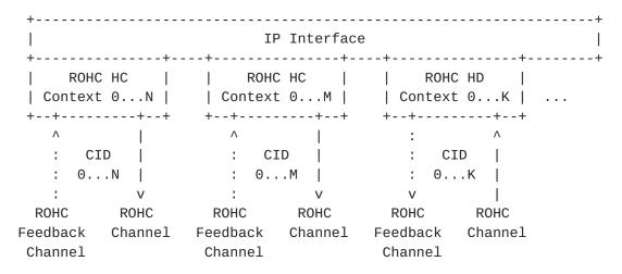
It should be noted that each ROHC instance at an IP interface therefore has its own context and CID space, and it must be ensured that the CID size of the corresponding decompressor at the other end of the ROHC channel is not smaller than the CID space of the compressor.
