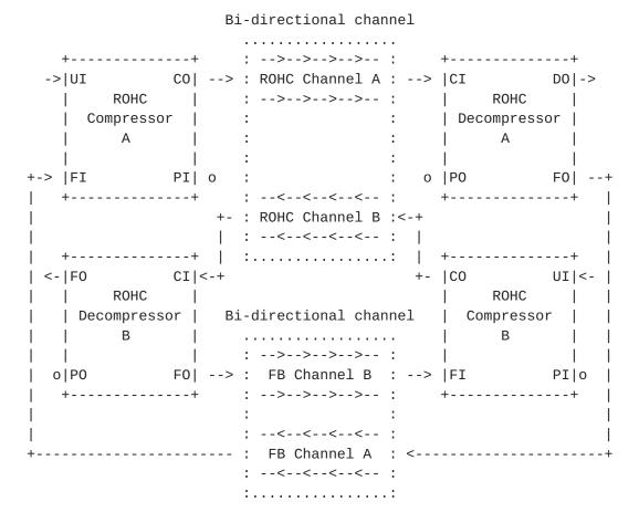
In this example, feedback is in both directions sent on its own dedicated channel, as discussed in e.g. feedback realization example 1-3 of ROHC [RFC-3095, page 44]. With this configuration, the piggybacking/interspersing mechanism of ROHC is not used, and the PI/PO connections are thus left open (marked with a "o"). It should be noted that in this picture also PO and FO at the decompressors have been swapped to simplify drawing, while the B-instances have been vertically mirrored.
