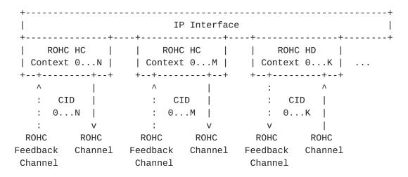
It should be noted that each ROHC instance at an IP interface therefore has its own context and CID space, and it must be ensured that the CID size of the corresponding decompressor at the other end of the ROHC channel is not smaller than the CID space of the compressor.
