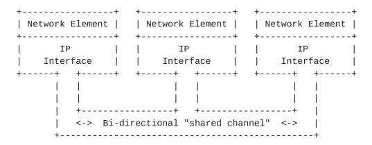
A typical example of a multipoint link with such a bi-directional "shared channel" is an Ethernet. Since the channel is shared, applying header compression would require a lower layer addressing scheme, to provide logical point-to-point channels, according to the definition of "channels".
