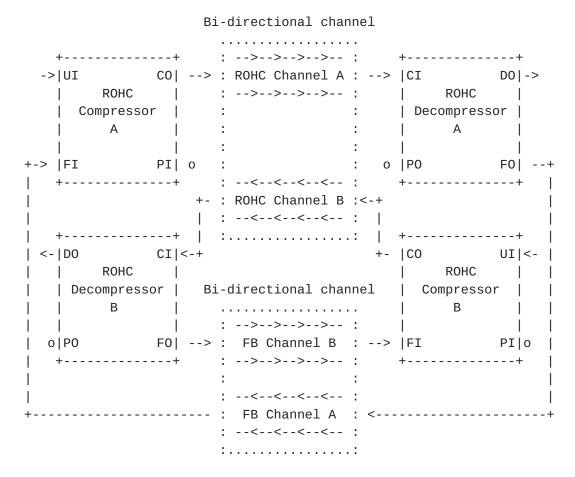
In this example, feedback is in both directions sent on its own dedicated channel, as discussed in e.g. feedback realization example 1-3 of ROHC [RFC-3095, page 44]. With this configuration, the piggybacking/interspersing mechanism of ROHC is not used, and the PI/PO connections are thus left open (marked with a "o"). It should be noted that in this picture FI/PI and PO/FO at the A-instances have been swapped to simplify drawing, while the B-instances have been horizontally mirrored.
