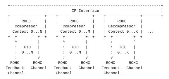
It should be noted that each ROHC instance at an IP interface therefore has its own context and CID space, and it must be ensured that the CID size of the corresponding decompressor at the other end of the ROHC channel is not smaller than the CID space of the compressor.
