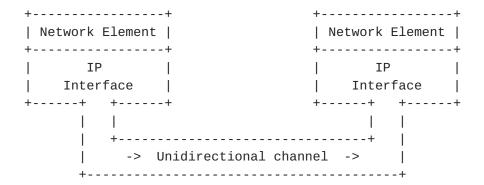
A typical example of a point-to-point link with one unidirectional channel like this is a satellite link. Since there is no return path present, only unidirectional header compression can be applied here.
