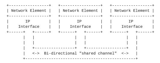
A typical example of a multipoint link with such a bi-directional "shared channel" is an Ethernet. Since the channel is shared, applying header compression would require a lower layer addressing scheme, to provide logical point-to-point channels, according to the definition of "channels".
