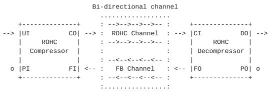
In this example, feedback is sent on its own dedicated channel, as discussed in e.g. feedback realization example 1-3 of ROHC [RFC-3095, page 44]. This means that the piggybacking/interspersing mechanism of ROHC is not used, and the PI/PO connections are thus left open (marked with a "o"). To facilitate communication with ROHC
