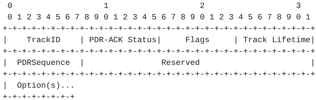
Figure 2: New PDR-ACK Control Message Format
