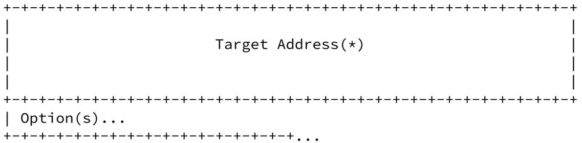
Figure 2: Format of the Discovery Reply Object (DRO)
