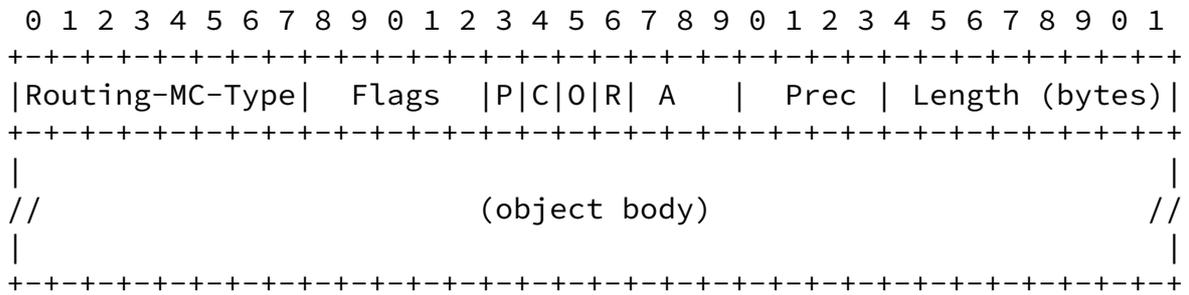
Figure 2: Routing Metric/Constraint object generic format
