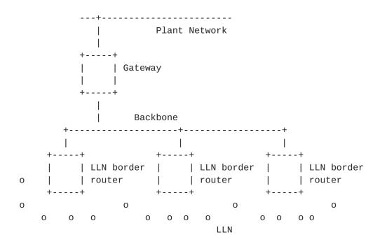
o : stationary wireless field device, seldom acting as an LLN router
