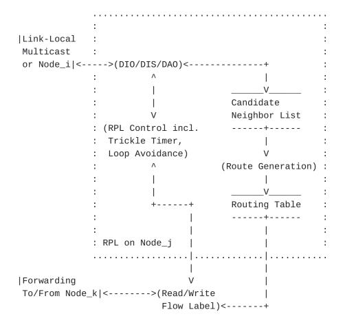
Figure 3: Data Flow Diagram of RPL
