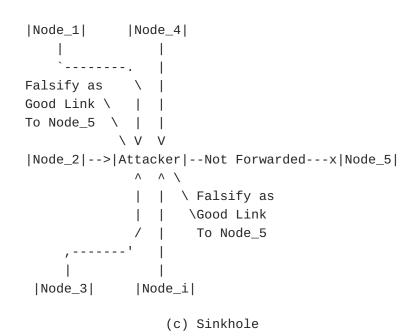
Figure 2: Selective Forwarding, Wormhole, and Sinkhole Attacks
