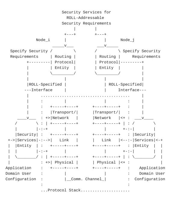
Figure 3: LLN Device Security Model
