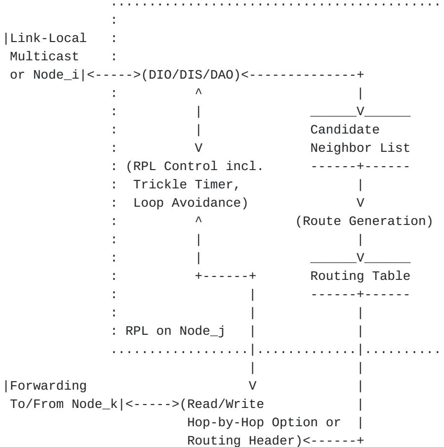
**Figure 4: Data Flow Diagram of RPL**
