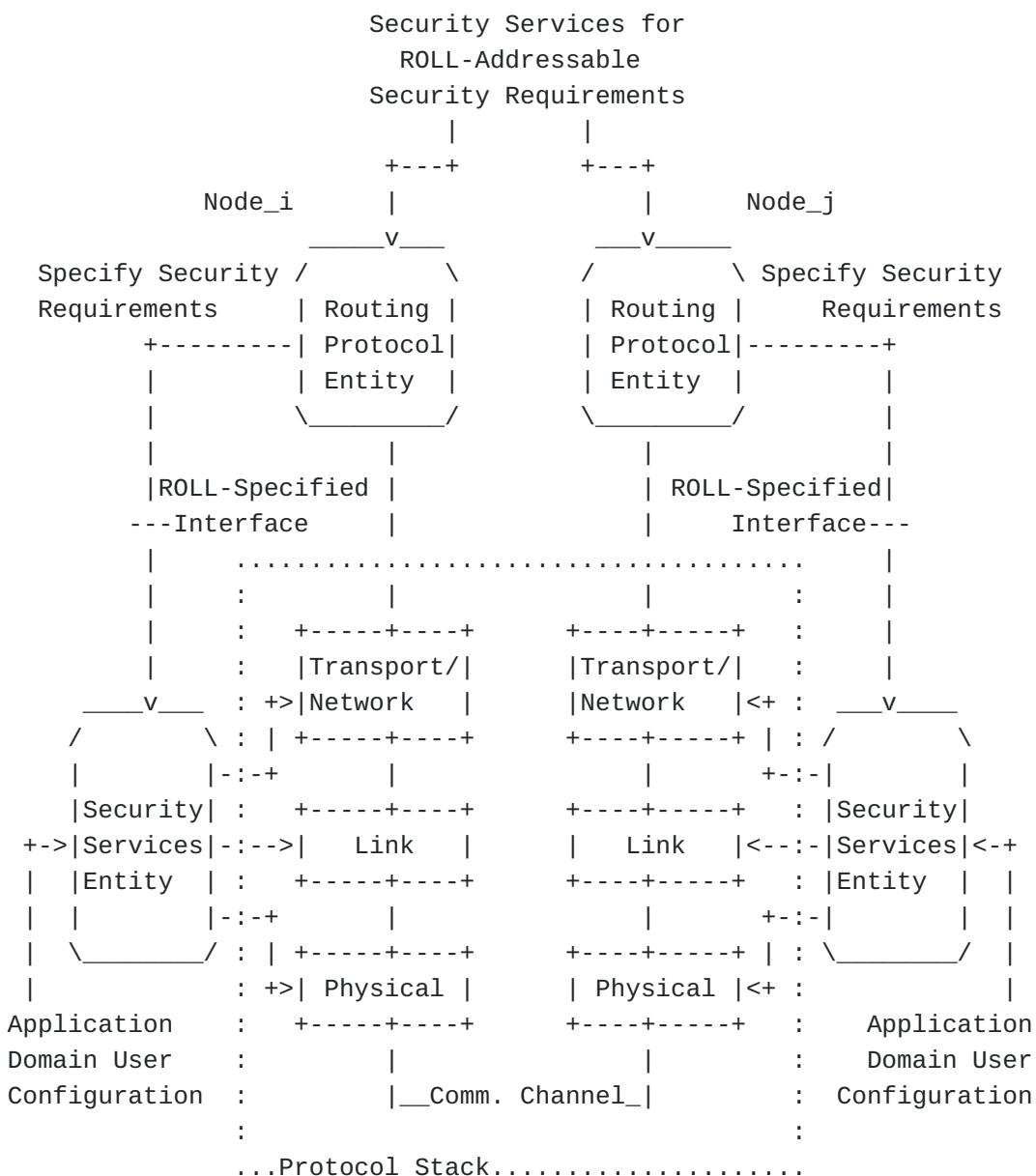
**Figure 3: LLN Device Security Model**
