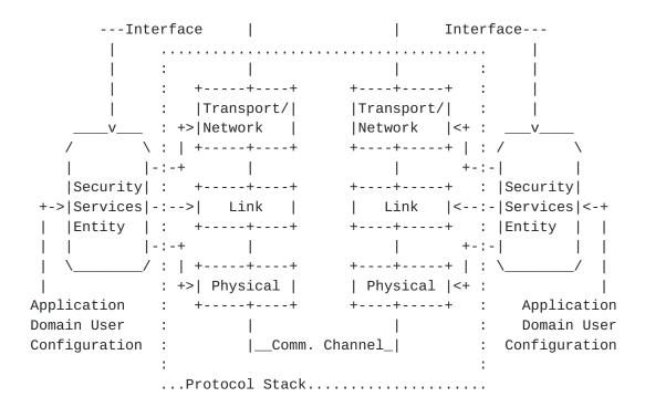
Figure 5: LLN Device Security Model
