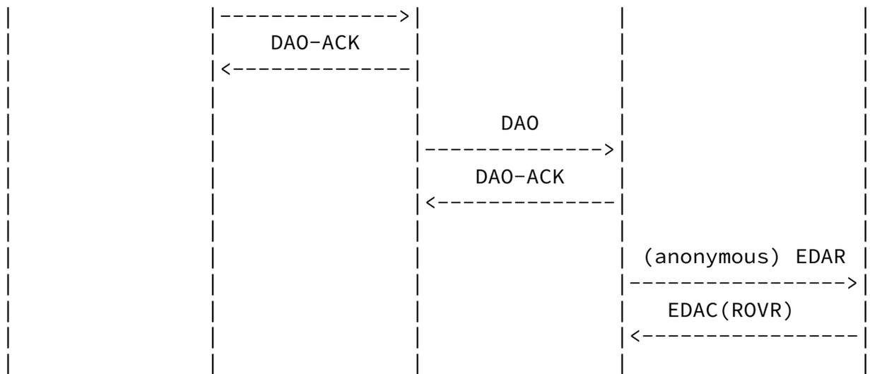
Figure 8: Next Registration Flow in Storing Mode
