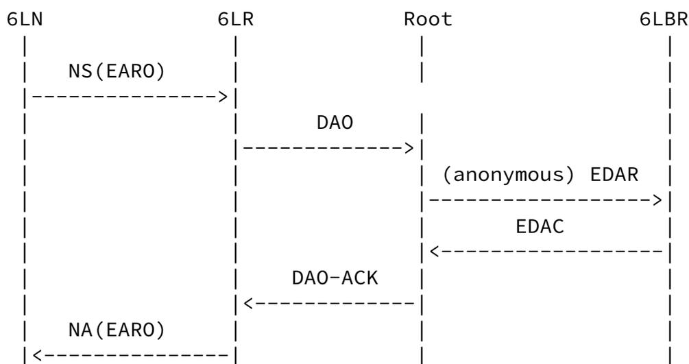
Figure 7: Next Registration Flow in Non-Storing Mode
