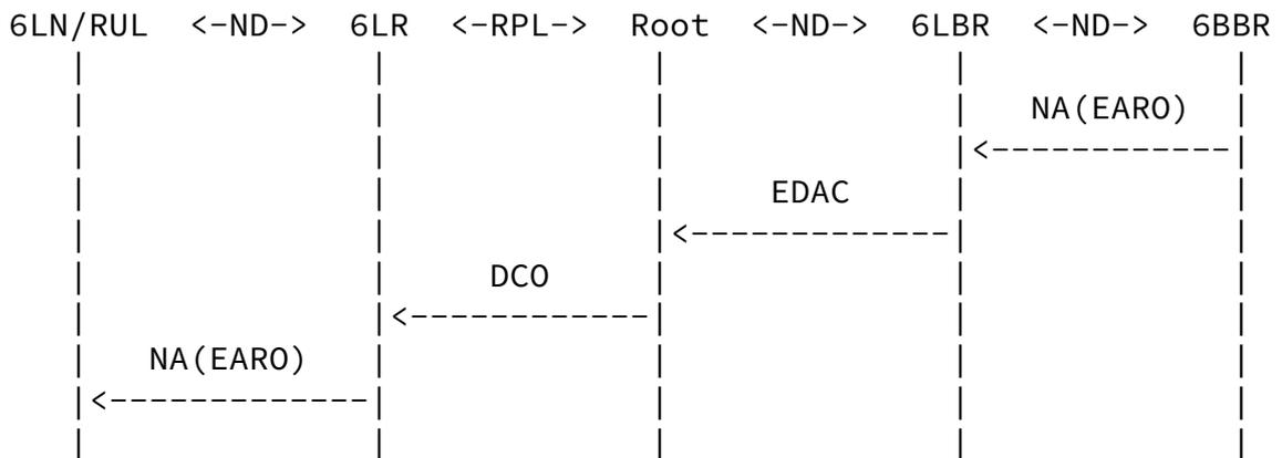
Figure 9: Asynchronous Issue
