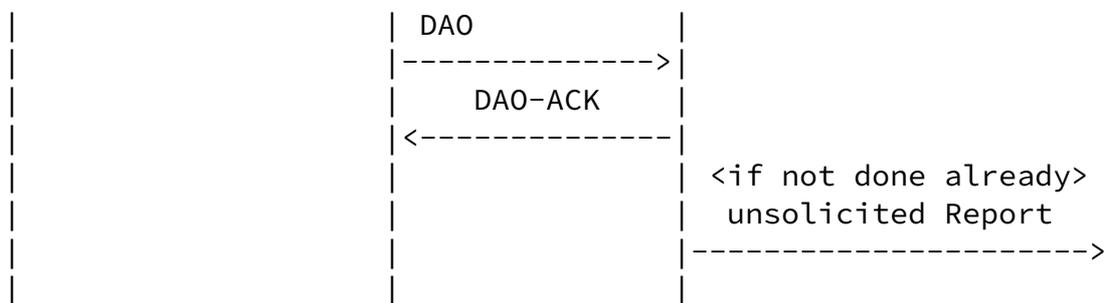
Figure 11: First Multicast Registration Flow
