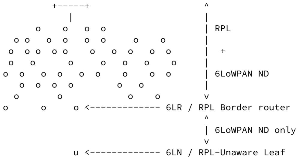
Figure 1: Injecting Routes on behalf of RULs
