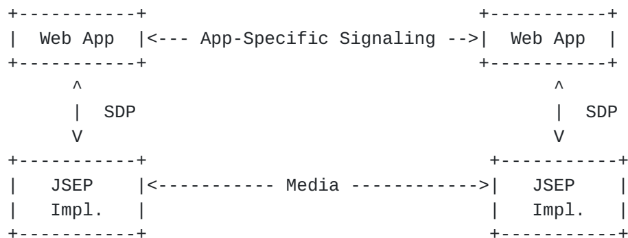
Figure 1: JSEP Signaling Model
