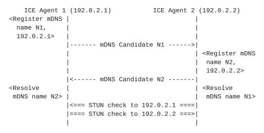
The exchange of ICE candidates relies on out-of-band signaling, for example, the SDP Offer/Answer procedure defined in [ICESDP]. In the above example, the candidate attributes in the SDP messages to exchange the mDNS candidates between ICE Agent 1 and 2 are as follows:
