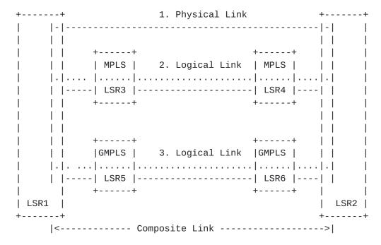
Figure 2: Illustration of Various Component Link Types
