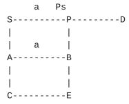
In some cases, it may be that the links comprising the SRLG occur in series on the path from S to the destination D, as shown in <a href="#Figure 5">Figure 5</a>. In this case, multiple consecutive repairs may be necessary. S will first repair to Ps, then P will repair to Dp. In both cases, because the links concerned are members of SRLG "a" the paths are computed to avoid all members of SRLG "a".
