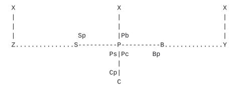
S should choose the closest router that can reach X during the failure as the alternate router. S determines which router to use as the alternate while running the SPF with P failed. This is accomplished by the normal process of re-attaching a leaf node to the core topology (this is sometimes known as a "partial SPF").
