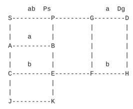
The link SP is a member of SRLGs "a" and "b". When a failure of the link SP is detected, it must be assumed that BOTH SRLGs have failed. Therefore the not-via path to Ps must be computed by failing all links which are members of SRLG "a" or SRLG "b". I.e. the semantics of Ps is now "P not-via any links which are members of any of the SRLGs of which link SP is a member". This is illustrated in <a href="Figure 8">Figure 8</a> below.
