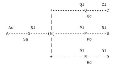
In this case, when S detected that P had failed it would send traffic reached via P and B to B not-via the LAN or any router attached to the LAN (i.e. to Bl). Any destination only reachable through P would be addressed to P not-via the LAN or any router attached to the LAN (except of course P).
