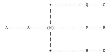
Consider the LAN shown in <u>Figure 10</u>. For connectivity purposes, we consider that the LAN is represented by the pseudonode (N). To provide IPFRR protection, S must run a connectivity check to each of its protected LAN adjacencies P, Q, and R, using, for example BFD [RFC5880].
