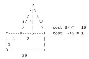
On failure of link XY, according to PLSN, S will regard R as a safe neighbor for traffic to D. However the ordered FIB rank of both R and T will be zero and hence these can change their FIBs during the same time interval. If R changes before T, then a loop will form around R, T and S. This can be prevented by using a stronger safety condition than PLSN currently specifies, at the cost of introducing more type C routers, and hence reducing the PLSN coverage.
