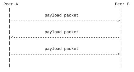
The third example is the first one that involves an actual REAP message. Here the hosts communicate in just one direction, so REAP messages are needed to indicate to the peer that sends payload packets that its packets are getting through:
