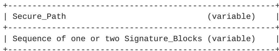
Figure 3: BGPsec_Path attribute format.
