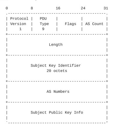
In addition to the normal boilerplate fields of an RPKI-Router PDU, the Router Key PDU has the following fields.
