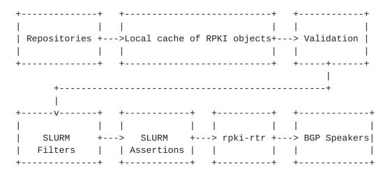
Figure 1: SLURM's Position in the Relying Party Stack
