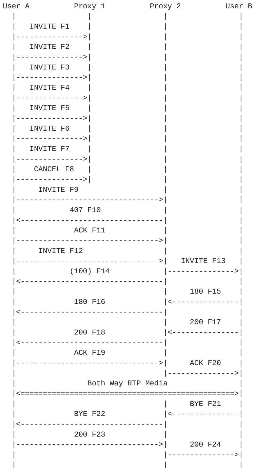
In this scenario, User A completes a call to User B via a Proxy Server. User A is configured for a primary SIP Proxy Server Proxy 1 and a secondary SIP Proxy Server Proxy 2 (Or is able to use DNS SRV records to locate Proxy 1 and Proxy 2). Proxy 1 is out of service and does not respond to INVITEs (it is reachable, but unresponsive). After sending a CANCEL to Proxy 1, User A then completes the call to User B using Proxy 2.
