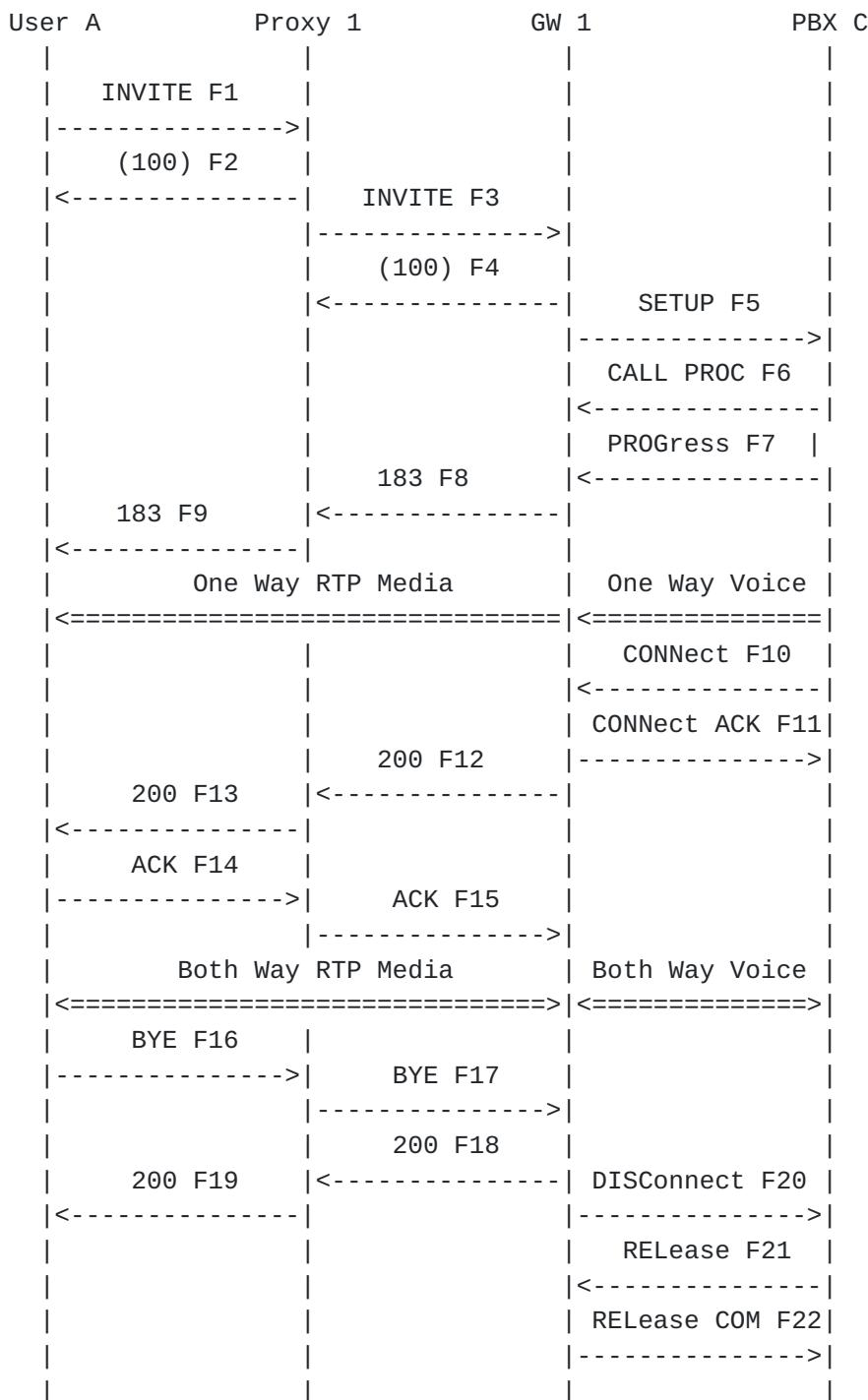
User A is a SIP device while User C is connected via an Enterprise Gateway (GW 1) to a PBX. The PBX connection is via a ISDN trunk group. User A dials User C's telephone number (918-555-3333) which is globalized and put into a SIP URL.
