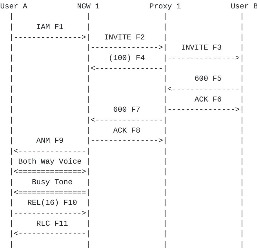
In this scenario, User A calls User B through Network Gateway NGW1 and Proxy 1. The call is routed to User B by Proxy 1. The call is rejected by the User B client. NGW 1 sets up a two way voice path to User A, plays busy tone, and releases call after timeout.
