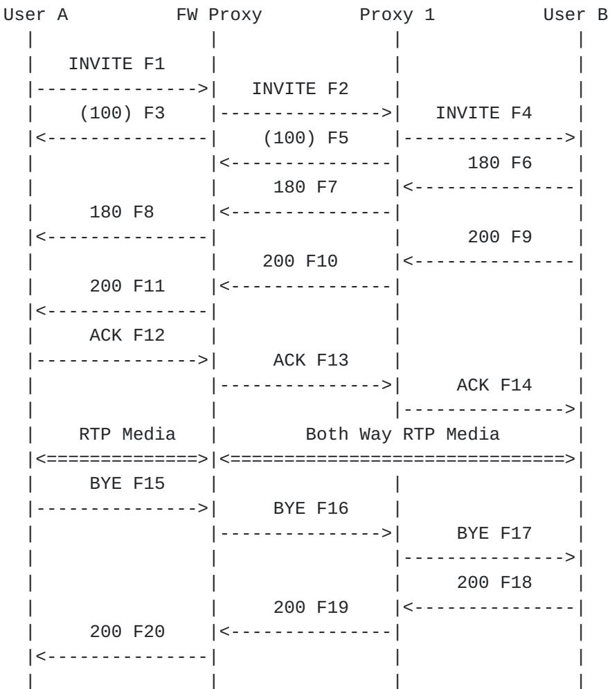
User A completes a call to User B through a Firewall Proxy and a SIP Proxy. The signaling message exchange is identical to 3.1.1 but the media stream setup is not end-to-end - the Firewall proxy terminates both media streams and bridges them. This is done by the Proxy modifying the SDP in the INVITE (F1) and 200 OK (F10) messages, and possibly any 18x or ACK messages containing SDP.
