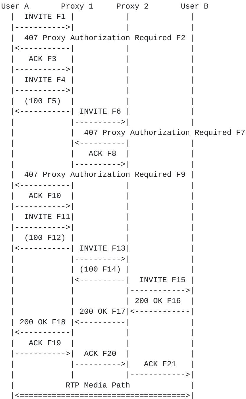
In this scenario, User A completes a call to User B using two proxies Proxy 1 and Proxy 2. The initial INVITE (F1) does not contain the Authorization credentials Proxy 1 requires, so a 407 Proxy Authorization response is sent containing the challenge information. A new INVITE (F4) is then sent containing the correct credentials and the call proceeds after Proxy 2 challenges and receives valid credentials. The call terminates when User B disconnects by
