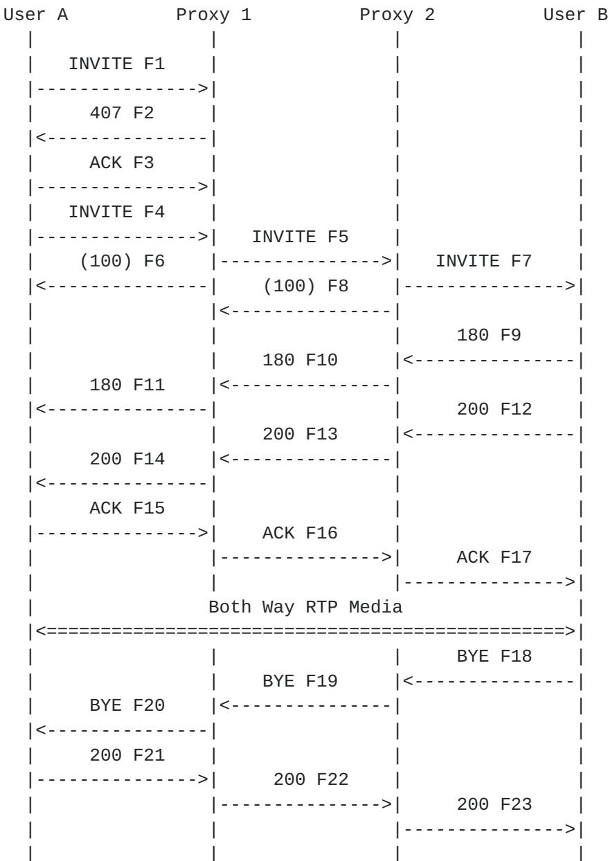
In this scenario, User A completes a call to User B using two proxies, Proxy 1 and Proxy 2. The initial INVITE (F1) does not contain the Authorization credentials Proxy 1 requires, so a 407 Proxy Authorization response is sent containing the challenge information. A new INVITE (F4) is then sent containing the correct credentials and the call proceeds. The call terminates when User B disconnects by initiating a BYE message.
