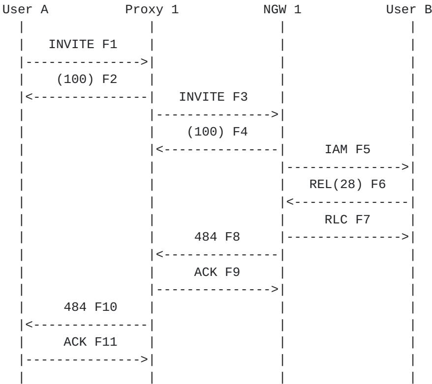
User A calls PSTN User B through a Proxy Server Proxy 1 and a Network Gateway NGW 1. However, User A does not provide enough digits for the call to be completed. The call is rejected by the PSTN with a ANSI ISUP Release message REL containing a specific Cause value. This cause value (28) is mapped by the Gateway to a SIP 484 Address Incomplete response which is proxied back to User A. For more details of ISUP cause value to SIP responses refer to [5].
