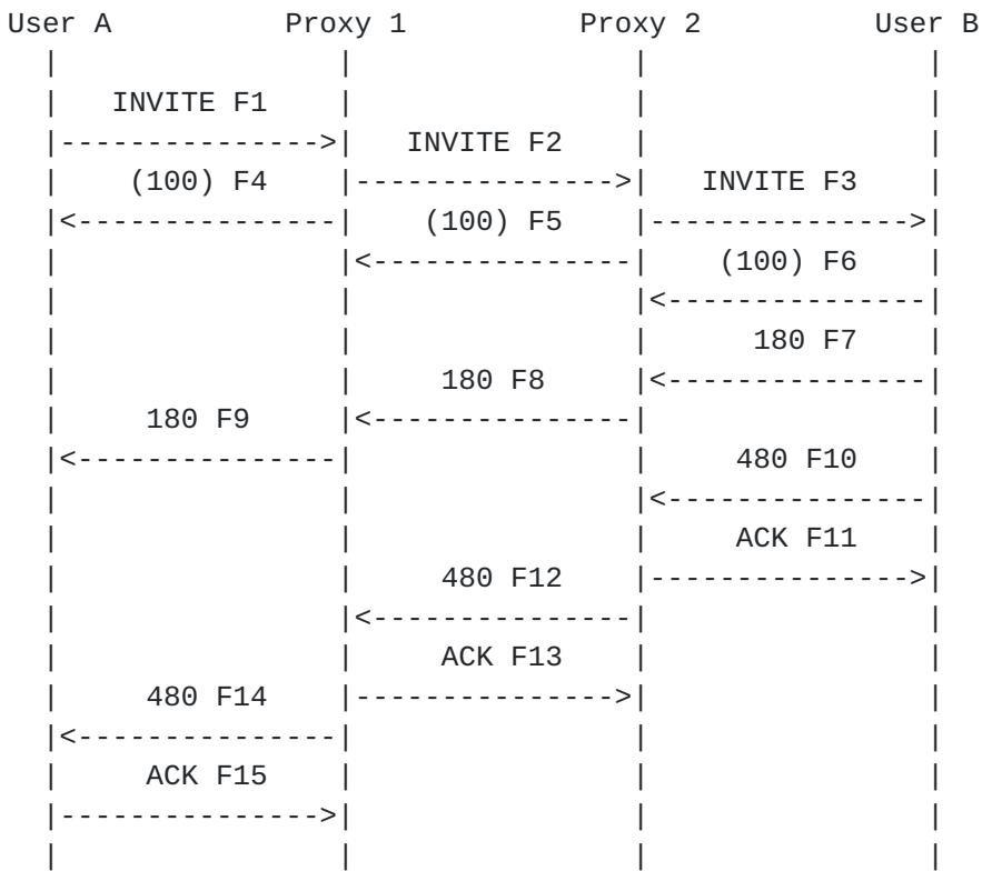
In this scenario, User B initially sends a 180 Ringing response to User A, indicating that alerting is taking place. However, then a 480 Unavailable is then sent to User A. This response is acknowledged then proxied back to User A.
