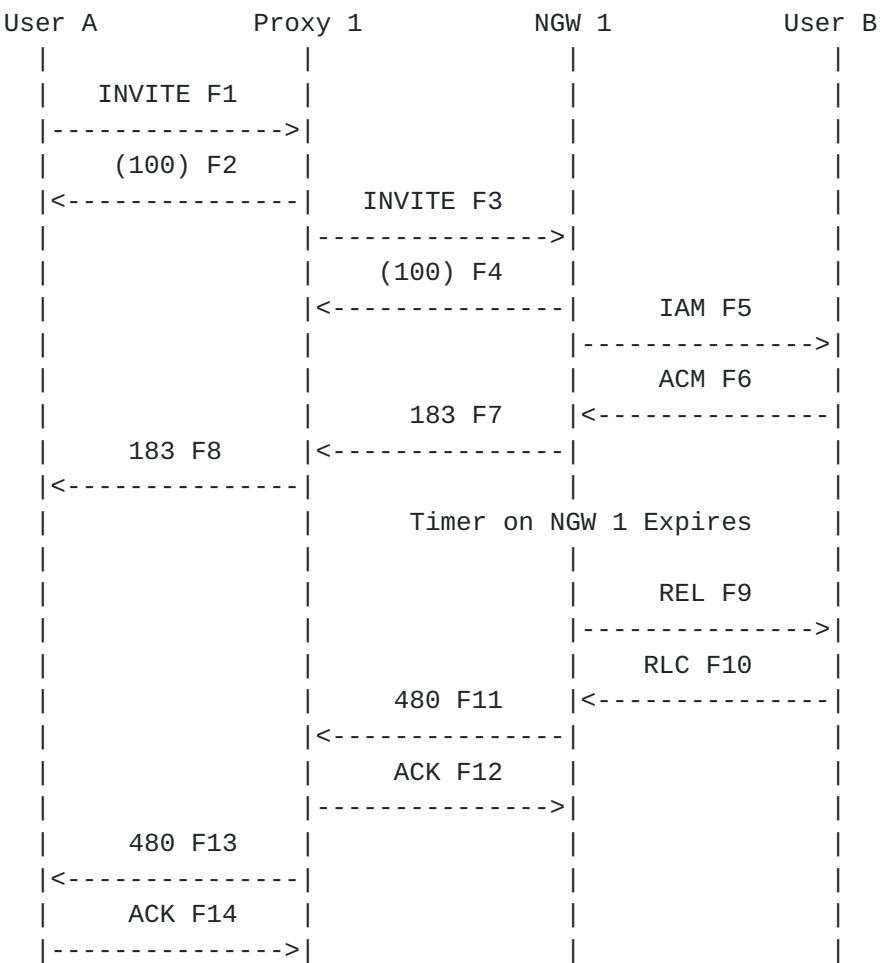
User A calls User B in the PSTN through a proxy server Proxy 1 and Network Gateway NGW 1. The call is released by the Gateway after a timer expires due to no ANswer Message (ANM) being received. The Gateway sends an ISUP Release REL message to the PSTN and a 480 Temporarily Unavailable response to User A in the SIP network.
