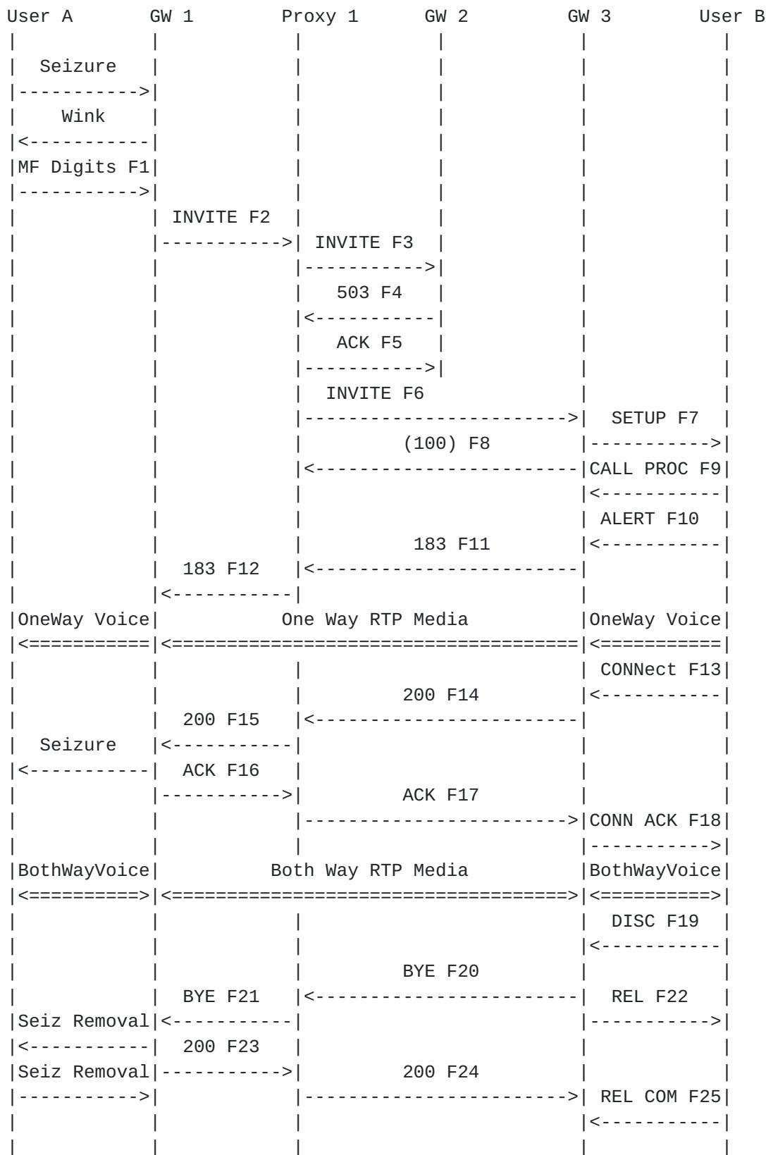
PBX User A calls PBX User C via Gateway GW 1 and Proxy 1. During the attempt to reach User C via GW 2, an error is encountered - Proxy 1 receives a 503 Service Unavailable (F4) response to the forwarded INVITE. This could be due to all circuits being busy, or some other outage at GW 2. Proxy 1 recognizes the error and uses an alternative route via GW 3 to terminate the call. From there, the call proceeds normally with User C answering the call. The call is terminated when User C hangs up.
