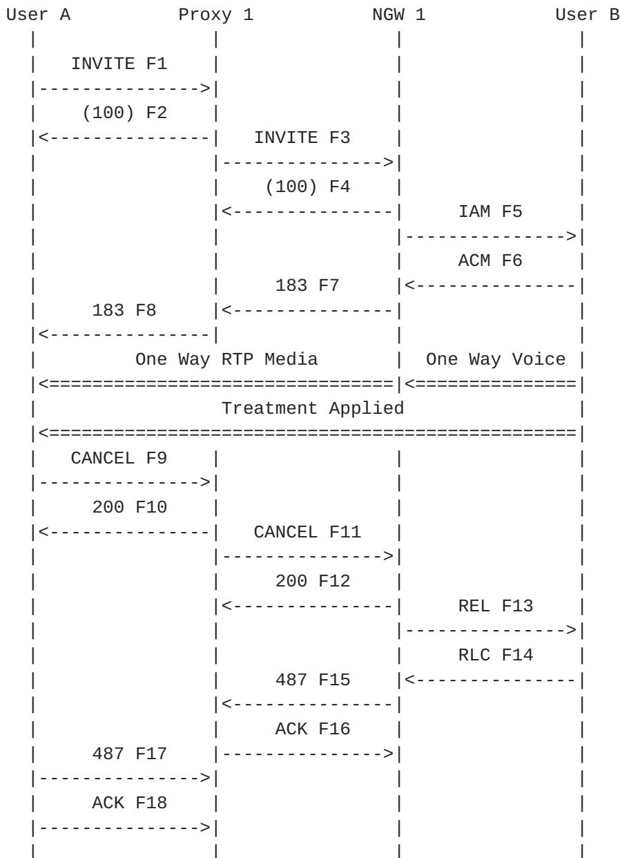
User A calls User B in the PSTN through a proxy server Proxy 1 and a Network Gateway NGW 1. The call is rejected by the PSTN with an in-band treatment (tone or recording) played. User A hears the treatment and then issues a CANCEL (F9) to terminate the call. (A BYE is not sent since no final response was ever received by User A.)
