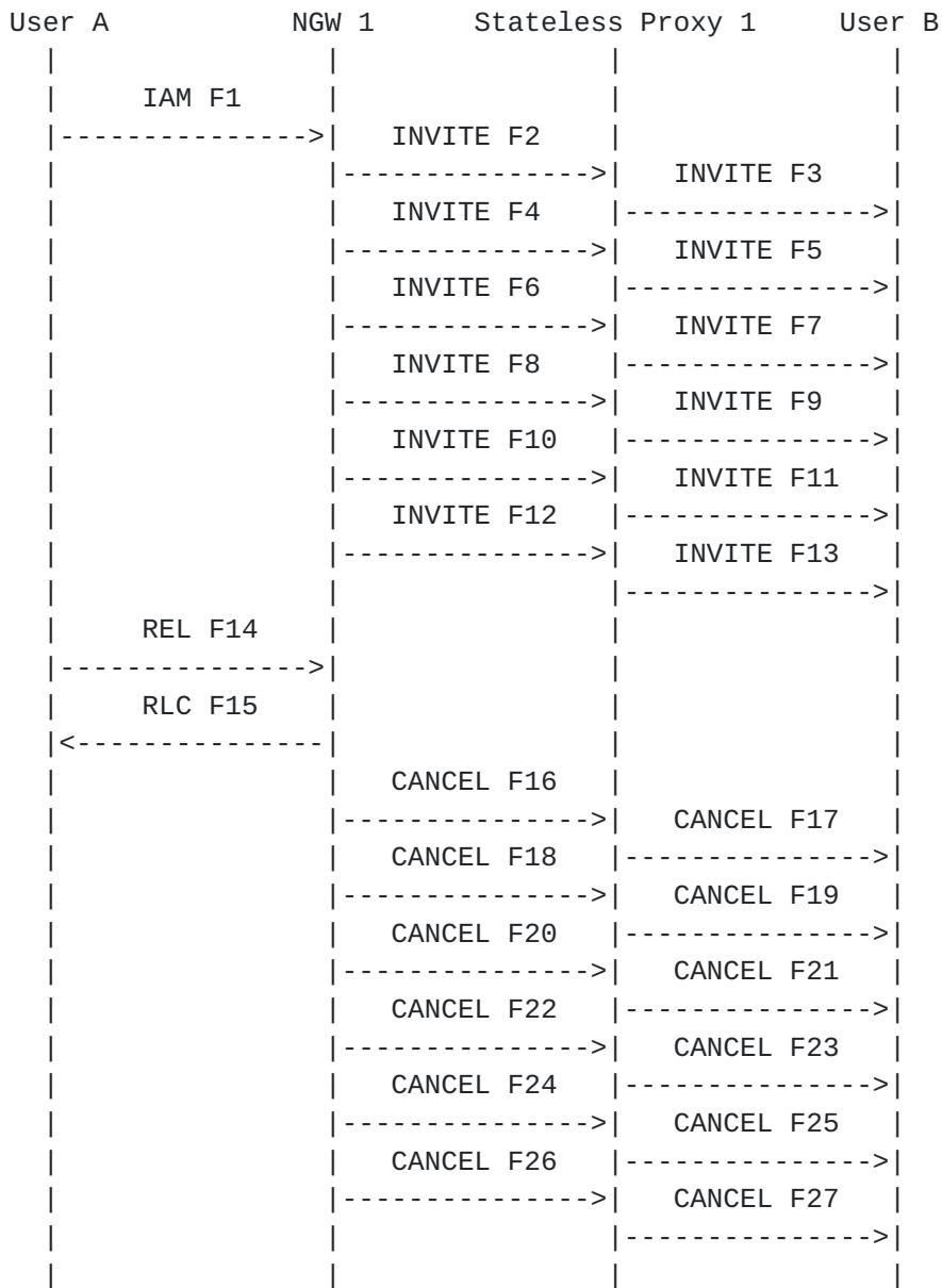
In this scenario, User A calls User B through NGW 1 and Proxy 1. Since Proxy 1 is stateless (it does not send a 100 Trying response), NGW 1 re-sends the INVITE and CANCEL messages after the expiration of SIP timer T1. User B does not respond with 180 Ringing. User A's network disconnects the call with a release REL (CauseCode=102 Timeout).
