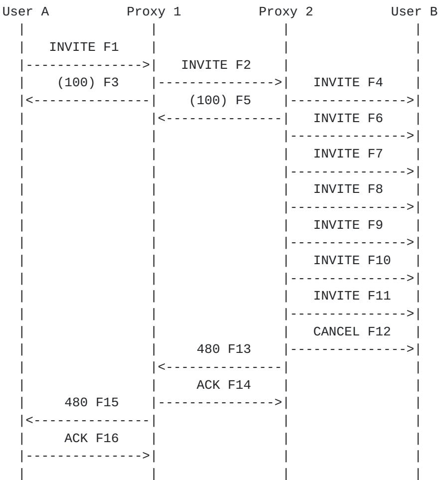
In this example, there is no response from User B to User A's INVITE messages being re-transmitted by Proxy 2. After the sixth re-transmission, Proxy 2 gives up and sends a CANCEL to User B and a 480 No Response to User A. Note that the CANCEL would also be retransmitted six times, as governed by SIP timer T1 as in Call Flow 5.2.6.
