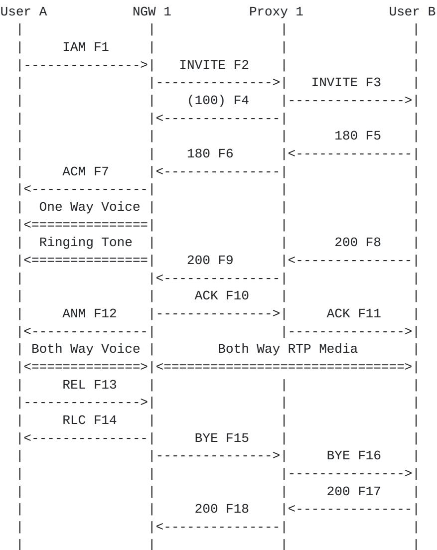
In this scenario, User A from the PSTN calls User B through a Network Gateway NGW1 and Proxy Server Proxy 1. When User B answers the call the media path is setup end-to-end. The call terminates when User A hangs up the call, with User A's telephone switch sending an ISUP RERelease message which is mapped to a BYE by NGW 1.
