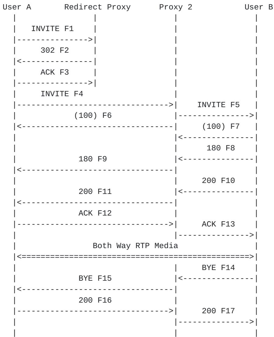
In this scenario, User A places a call to User B using first a Redirect server then a Proxy Server. The INVITE message is first sent to the Redirect Server. The Server returns a 302 Moved Temporarily response (F2) containing a Contact header with User B's current SIP address. User A then generates a new INVITE and sends to User B via the Proxy Server and the call proceeds normally. In this example, no SDP is present in the INVITE, so the SDP is carried in the ACK message.
