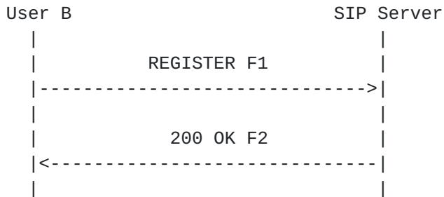
User B sends a register request to the Proxy Server containing no Contact headers, indicating the user wishes to query the server for the user's current contact list. Since the user already has authenticated with the server, the user supplies authentication credentials with the request and is not challenged by the server. The SIP server validates the user's credentials. The server returns a response (200 OK) which includes the user's current registration list in Contact headers.
