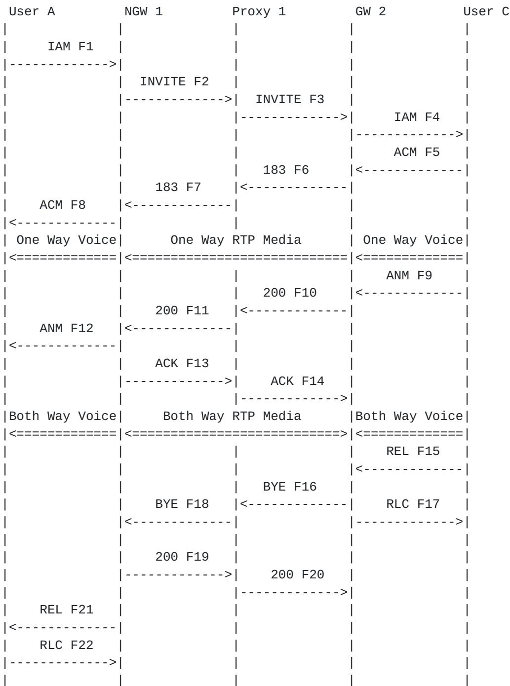
In this scenario, User A in the PSTN calls User C who is an extension on a PBX. User A's telephone switch signals via SS7 to the Network Gateway NGW 1, while User C's PBX signals via SS7 with the Enterprise Gateway GW 2. The CdPN and CgPN are mapped by GW1 into SIP URLs and placed in the To and From headers. Proxy 1 looks up the dialed
