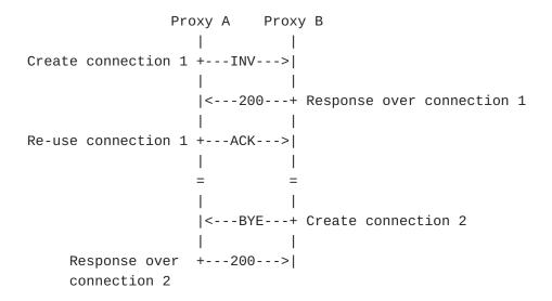
Figure 3: Multiple connections for requests
