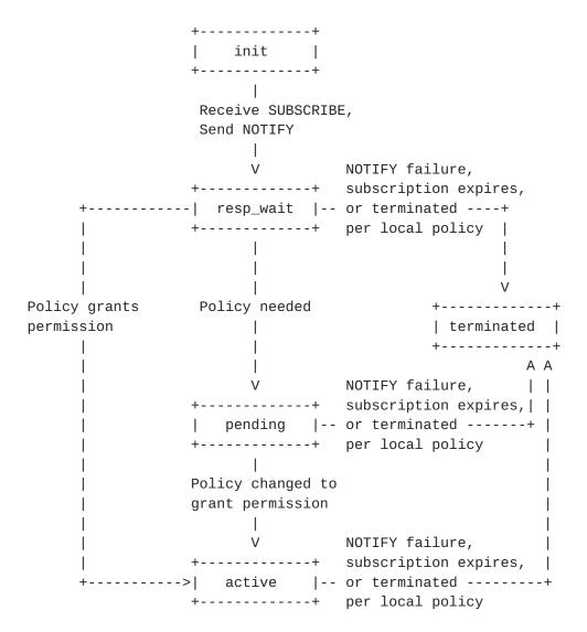
When a SUBSCRIBE request is answered with a 200-class response, the notifier MUST immediately construct and send a NOTIFY request to the subscriber. When a change in the subscribed state occurs, the notifier SHOULD immediately construct and send a NOTIFY request, subject to authorization, local policy, and throttling considerations.
