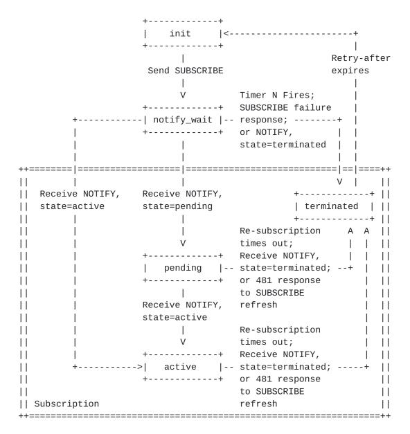
In the state diagram, "Re-subscription times out" means that an attempt to refresh or update the subscription using a new SUBSCRIBE request does not result in a NOTIFY request before the corresponding Timer N expires.
