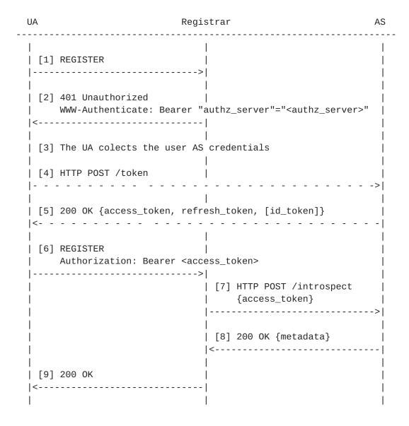
In step [1], the UA starts the registration process by sending a SIP REGISTER request to the registrar without any credentials. The REGISTER request includes an indication that the UA supports tokenbased autentication, using a sip.token media feature tag.
