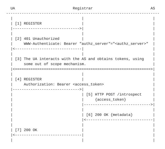
In step [1], the UA starts the registration process by sending a SIP REGISTER request to the registrar without any credentials. The REGISTER request includes an indication that the UA supports tokenbased autentication, using a sip.token media feature tag.
