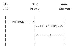
Figure 1: Call flow over the SIP-AAA interface
