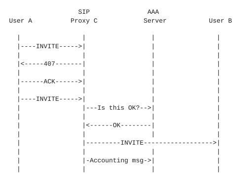
Figure 2: WLAN roaming user
